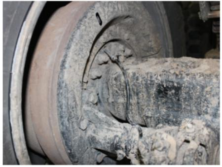
Excess wire length should be coiled appropriately (loops no smaller than 10 cm in diameter) and secured with tie wraps in a safe location.
