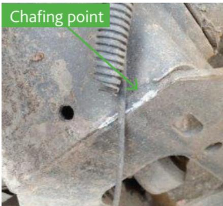
The cable routing and length must accommodate full suspension travel.
