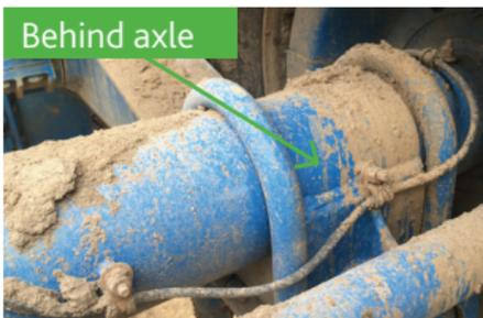
Use grommets or other protection for wires passing through metallic frame members.
