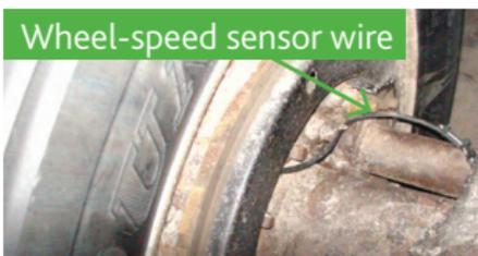
Ideally, this wire should be located on the top side of the axle (rearward of travel direction).
