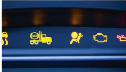
When using the blink code method on some systems, each fault must be addressed before further faults can be diagnosed.
