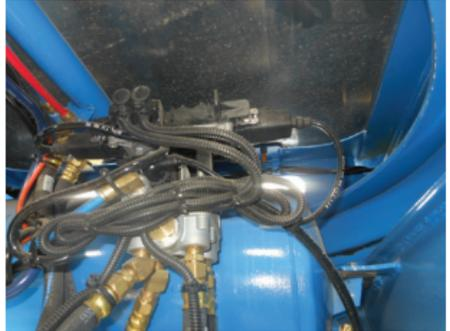
Where possible, replace extension wires with appropriate length to minimize the amount of coiling required.
